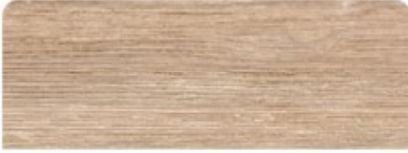
a-Step: The special color that is achieved by applying and brushing a water-based semi-opaque paint on top of a low-resin white patina paint.
