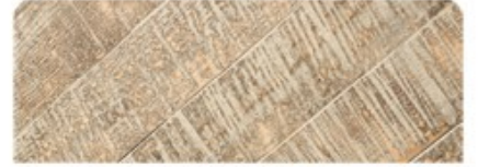
c-Ganita: Water-based semi-opaque paint is applied on top of water-based covering paint. After the drying process is completed, it is cleared using low-grit sandpaper to achieve a special color.
